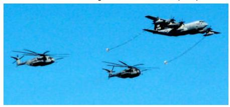
Two Marine helicopters are hooking up for refueling.
