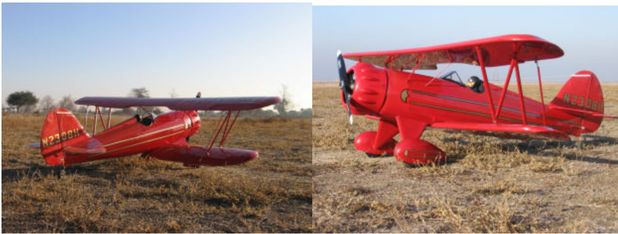
Walt's Cloers WACO YMF-5, Pica kit, (?) wingspan, 1/6 scale, 10 lb. Motor: AXI 4130/14 Batteries: (2) 11.1 V , Propeller: 16/10.
