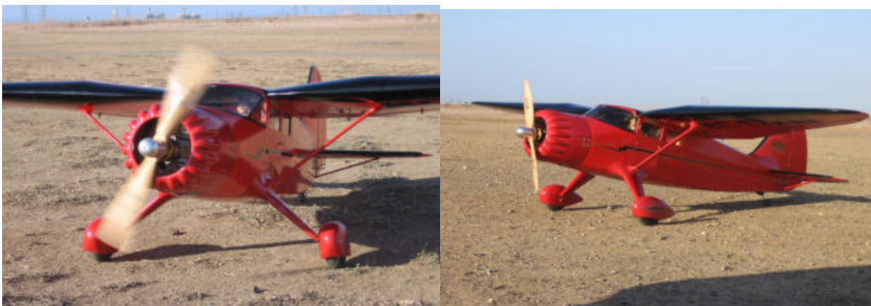
Don Holfelt's Stinson SR-9 s from the Top Flite 100" wingspan, 9.5 lb., Motor: AXI 5330/24, Batteries: 10 cell LiPoly.
